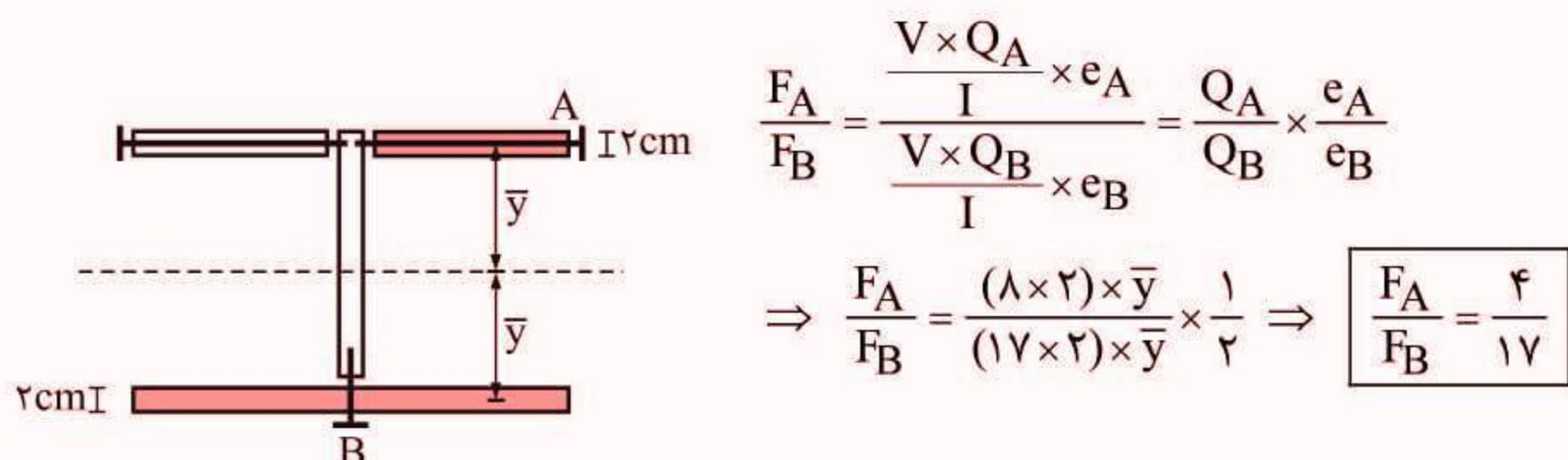
$$\frac{F_A}{F_B} = \frac{\frac{V \times Q_A}{I} \times e_A}{\frac{V \times Q_B}{I} \times e_B} = \frac{Q_A}{Q_B} \times \frac{e_A}{e_B}$$
