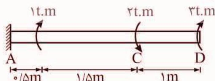
$$\phi_D = \sum \frac{T_i L_i}{GJ} = \frac{1 \times 0.15}{55} - \frac{2 \times 2}{55} + \frac{3 \times 3}{55} = \frac{5/5}{55} = 0.1 \text{ rad} = 0.1 \times \frac{180}{\pi} = \frac{18}{\pi} = 5.47^\circ$$
