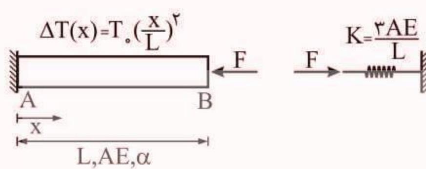
$$\begin{aligned}\vec{\Delta}_B &= \Delta L \Rightarrow \int_0^L \alpha \Delta T(x) dx - \frac{FL}{AE} = \frac{F}{\frac{3AE}{L}} \\ &\Rightarrow \int_0^L \alpha T_0 \left(\frac{x}{L}\right)^3 dx = \frac{FL}{3AE} \Rightarrow \frac{\alpha L T_0}{3} = \frac{FL}{3AE} \\ &\Rightarrow F = \frac{1}{4} AE \alpha T_0\end{aligned}$$
