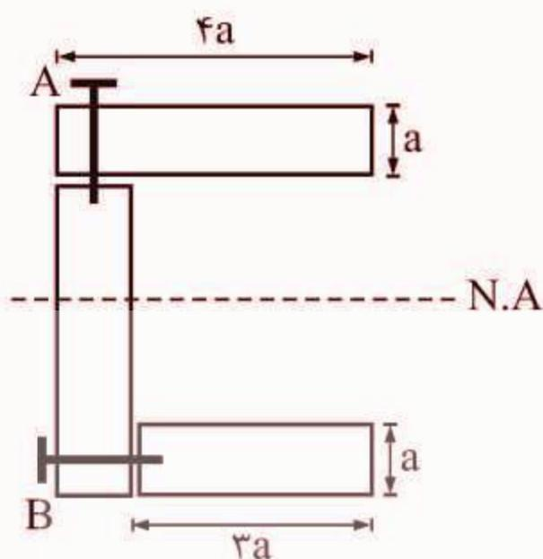
$$\frac{F_A}{F_B} = \frac{\frac{V \times Q_A}{I} \times e_A}{\frac{V \times Q_B}{I} \times e_B} = \frac{Q_A}{Q_B} \times \frac{e_A}{e_B}$$
