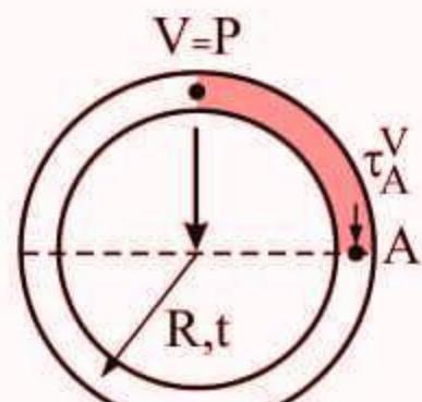
$$\tau_A^V = \frac{V}{I} \times Q = \frac{P}{\pi R^3 t} \times \frac{\frac{\pi}{2} R t \times \frac{2R}{\pi}}{t} = \frac{P}{\pi R t}$$
